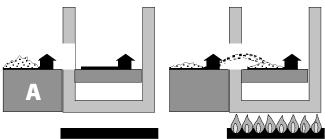
AB. As grain is pitched onto the elevator, heat is added to the gas. The elevator does not move up, but the pressure quadruples.
