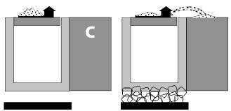
CD. Once the piston reaches the high elevation, the heat is turned off. As grain is pitched off the elevator, the gas is cooled. During this process, the pressure is reduced to its original value.
