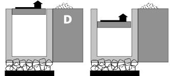
DA. Once the grain is offloaded, continued cooling of the gas causes the piston to fall. During this process, the volume of the gas returns to its original value. This takes the gas to its original state.
