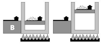
BC. Once the grain is fully loaded, the elevator door is shut. Heat added to the gas now causes the piston to rise. During this process, the volume of the gas triples.
