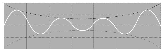
4. What kind of sound would produce the pattern (trace) shown above? (The dashed line represents the amplitude envelope and therefore shows the variation in volume.)
