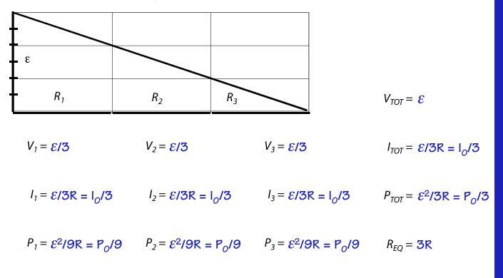
4. Unequal Runs  $(R_2 = 3R_1; R_1 = R)$  (this time, you draw in the V's and I's)
