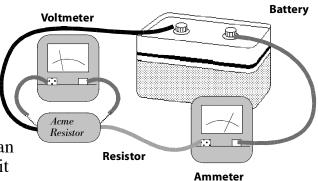
If a 6 volt potential induces a current of 2 amperes, the conductor has a resistance of 3 ohms.
